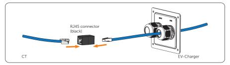
Figure 6-26 Using RJ45 connector
