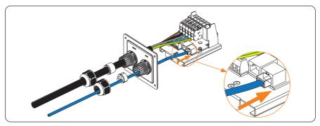
Figure 6-28 Connect the communication cable to RJ45 port
