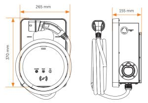
Figure 2-6 Dimensions of Plug Type
