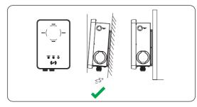
Figure 6-1 Correct installtion
