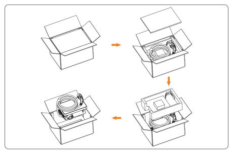
Figure 5-2 Unpacking the Plug Type EV-Charger
