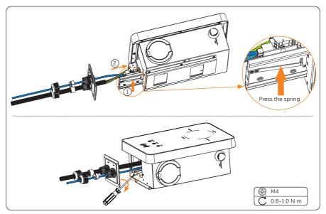
**Step 12**: Press the spring upward and push the base plate of communication board in. Then screw the countersunk screw.
