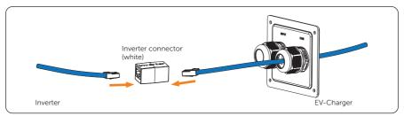
Figure 6-30 Using the white inverter connector
