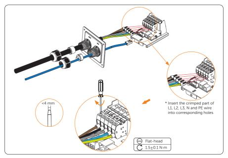
Figure 6-22 Connect the AC input cable
