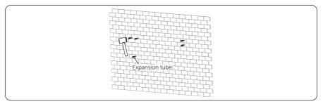
Figure 6-10 Insert the expansion tubes
