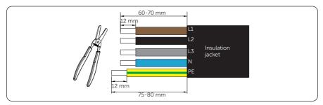
Figure 6-14 Strip the AC input cable
