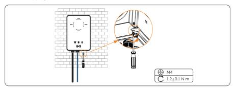
Figure 6-34 Hang and steady the EV-Charger
