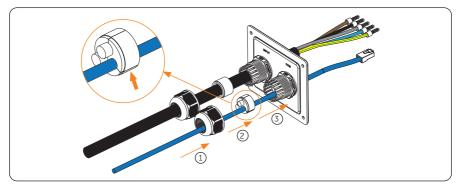
Figure 6-21 Thread the communication cable
