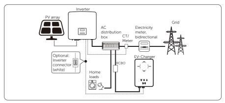
Figure 6-4 Home scene and communication with inverter
