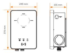
Figure 2-5 Dimensions of Socket Type
