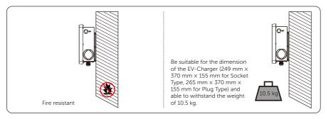
Figure 4-1 Installation carrier requirement
