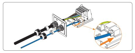
Figure 6-24 Connect the communication cable to RJ45 port
