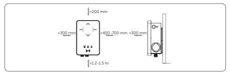
Figure 4-2 Clearance requirement
