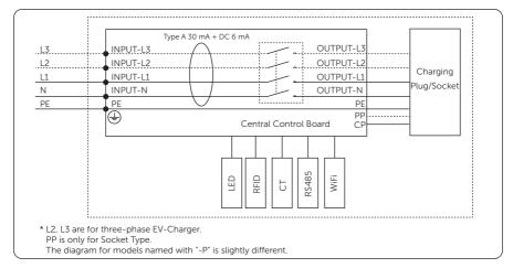
Figure 2-8 Principle Circuit Diagram
