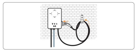
For Plug Type, connect the charging connector with the EV-Charger and hang the connecting cable on the cable hook.
