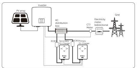
Figure 14-3 Parallel function - communication with inverter
