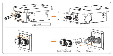
Figure 6-12 Take down and dissassemble the rear cover
