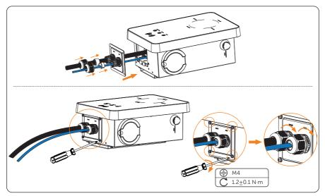
Figure 6-33 Secure the rear cover
