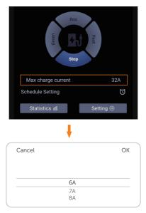
Figure 9-25 Setting max charging current
