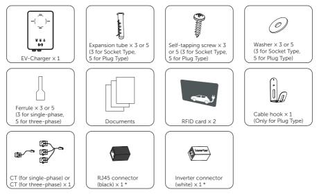
\* The black RJ45 connector is for extension connection of CT or network, while the white inverter connector is specially supplied for connecting inverter.
