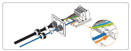
Figure 6-31 Connect the communication cable to Network port
