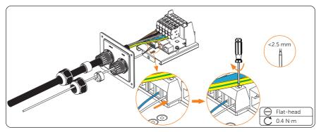
Figure 6-27 Connect the communication cable to RS485 port
