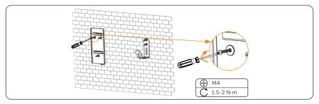
Figure 6-11 Secure the bracket and the cable hook
