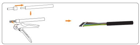
Figure 6-15 Crimp the wires
