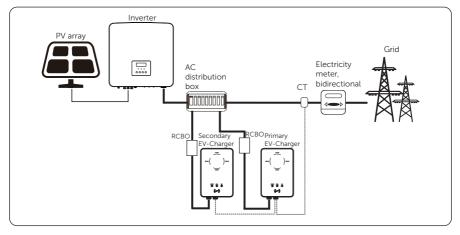
Figure 14-4 Parallel function - communication with CT
