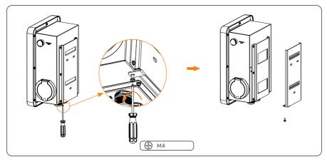
Figure 6-7 Remove the back bracket away
